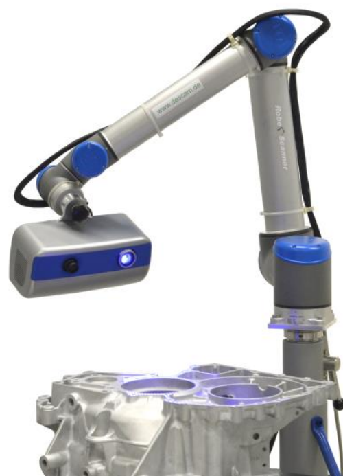
RoboScanner measuring a gear box
