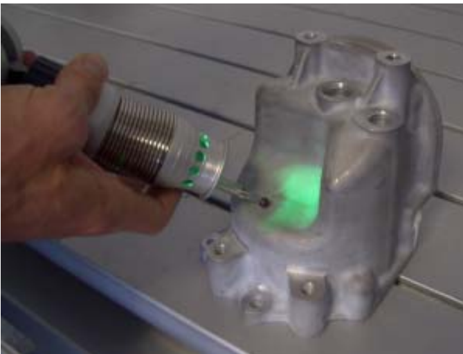
Photo 2: Operating the floating probe of the MCA.
