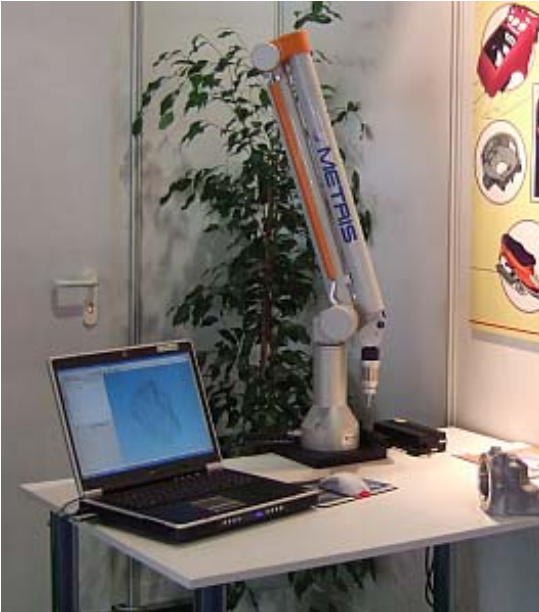
Photo 1: 6 axes MCA measurement arm.
