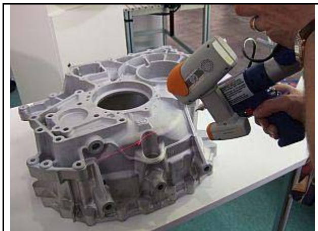
DESCAM's new ModelMaker D handheld scanner features a wide scan stripe measuring 180mm.
