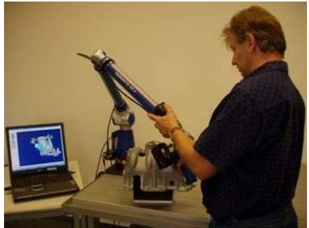
Laser scanning of a manifold
