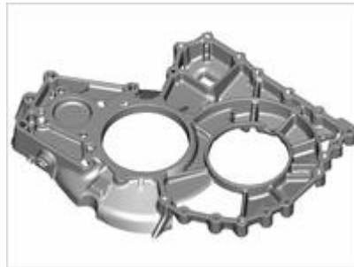
Scan data of the surface of the gearbox
